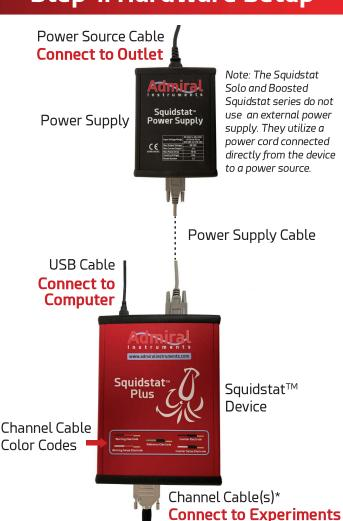
\*The Squidstat Prime, Squidstat Cycler, and Boosted Squidstat models have channel cable connections with multiple cables different from this diagram.
