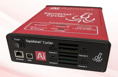
24-bit A/D converter for 0.06 parts-per-million resolution
